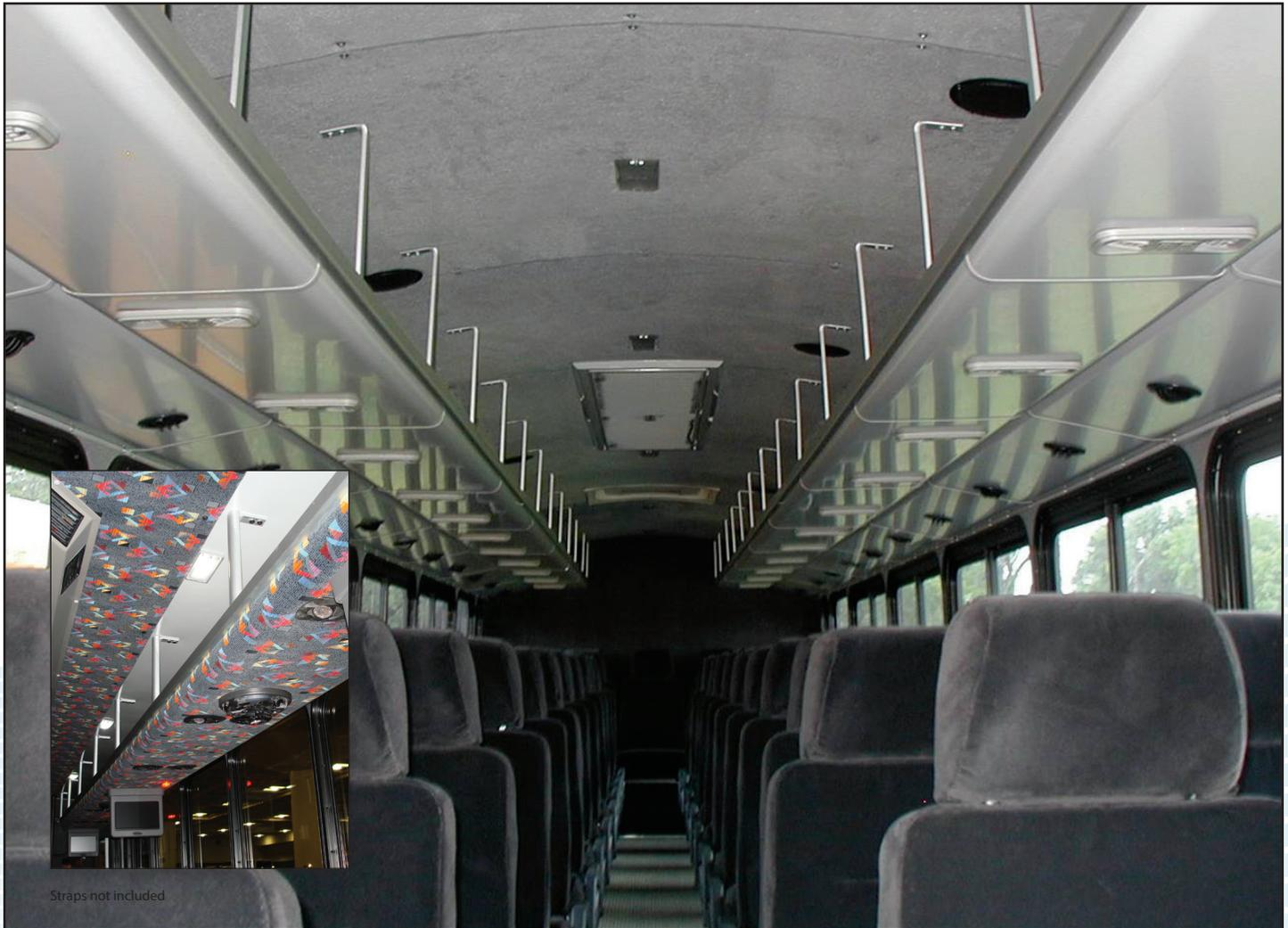
Designed and manufactured for each individual bus model providing unique and cost effective solutions. Pretoria pioneered the use of lightweight aluminum composite panels in conjunction with satin anodized aluminum extrusions to provide solid and easy to install systems. All of our OPR's systems are available with integral ducting that is engineered for use with all types of AC units.
