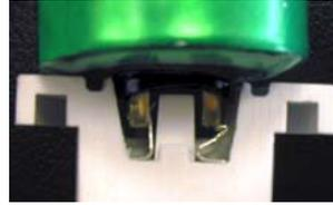
Damaged RDC & Damaged Socket Receptacle
