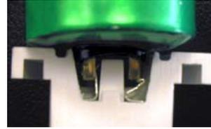
Damaged RDC & Damaged Socket Receptacle
