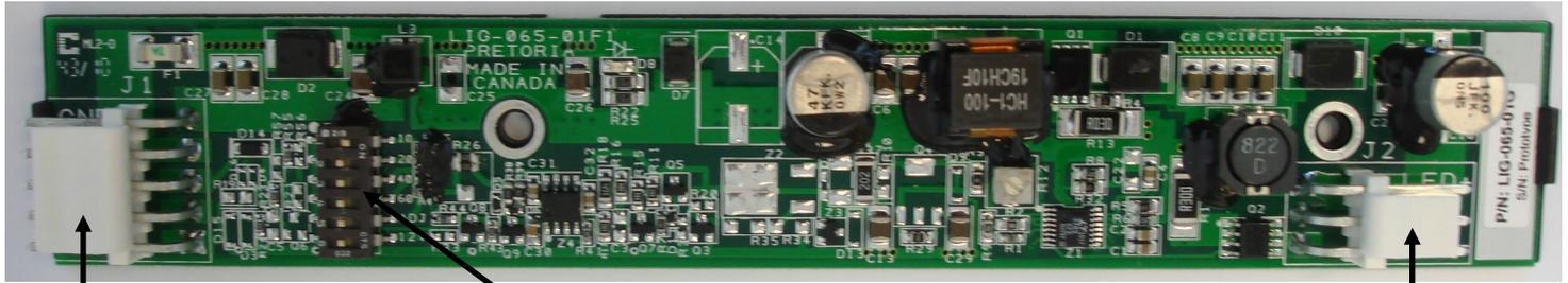
Input connector from bus to LED driver
