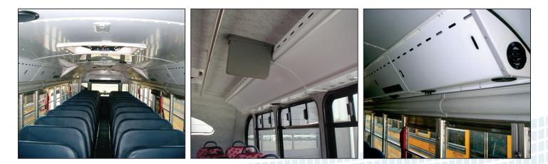
Our design team works closely with the bus OEM, the AC OEM and the customer to provide air moving systems that are both functional and aesthetically pleasing. For example, our vacuum forming and mold construction processes ensure the ABS end caps provide an excellent "fit and finish".
