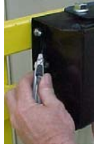
2. Cut seal at both ends of cover.
