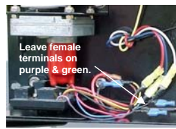
28. Tie wires. View of completed internal installation. Note: Purple & green wires from module not used - insulate & tie with other wires -do not remove female terminals installed on ends.
