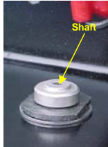
14. Close-up of shaft, bushing & washer installed.
