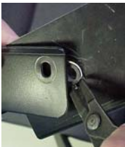
13. Install new spring clip in plastic bushing groove.
