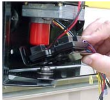
23. Hold motor wires. Insert module assembly at an angle to clear motor.
