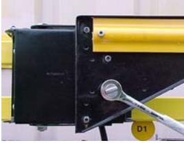
1. Remove (4) 1/4-20 nuts with 7/16" wrench & remove arm.
