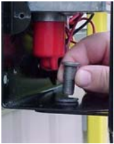
9. Remove hinge pin. Discard.
