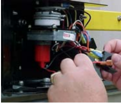
18. Disconnect -double red, single red & double white from lower relay; -double blue/green & black from upper relay.
