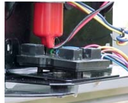
24. Set module on shaft - rotate bushing as reqd for module to set evenly. Align w/holes in box. (Drill 9/32 hole if mntg. brkt. interferes.)
