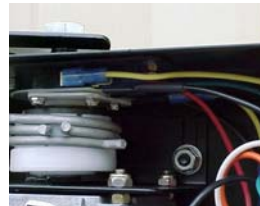
20. Remove yellow, brown & green from rear micro-switch; yellow & red from front switch. Discard relays.
