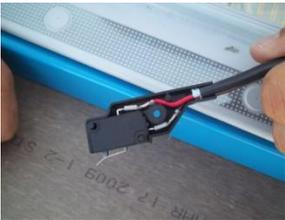
Switch removed from hatch
