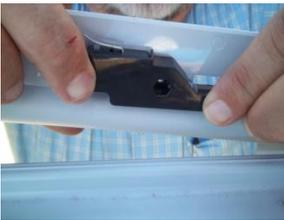
Reinstall switch by aligning locator tabs on switch cover to holes on release hinge
