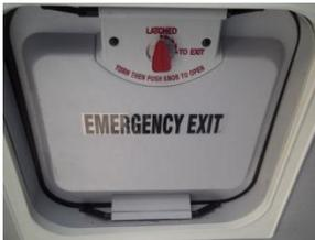
Close hatch and rotate knob to latched position.
