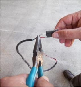
Using needle nose pliers remove top connector
