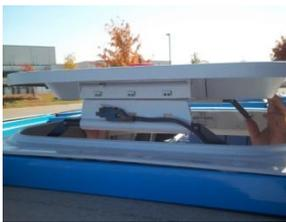
Lower hatch down and onto release hinge
