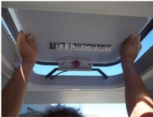
Lift hatch to normal venting position
