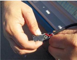
Separate switch and pigtail from switch cover
