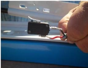
Switch prepared for installation, note wire locations, longer wire on bottom connector, and shorter wire on top connector
