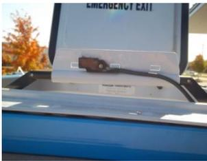
Switch mounted and secured to release hinge
