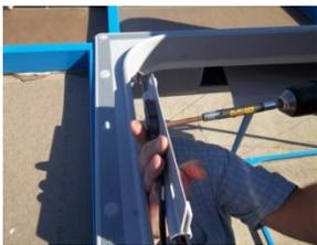
Put one finger over hole in back of screw to keep the hex nut captured while removing.
