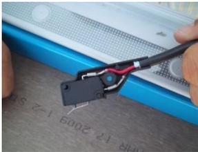
Switch removed from hatch
