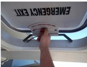
Place hatch lever to open position
