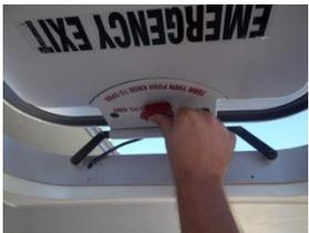
Push the button on hatch knob to open hatch
