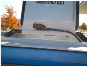
Switch mounted and secured to release hinge
