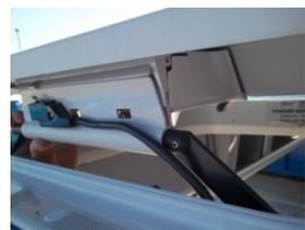
Insure hatch is seated properly onto release hinge
