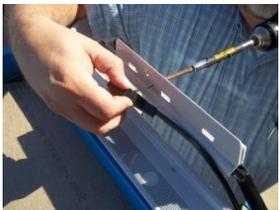
At this point the old switch and cover should fall when the hex nut is loosened
