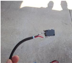
The pigtail is attached to the switch by spade connectors
