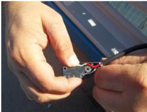
Separate switch and pigtail from switch cover
