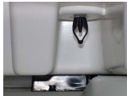
New Rivet (inside view of lid)
