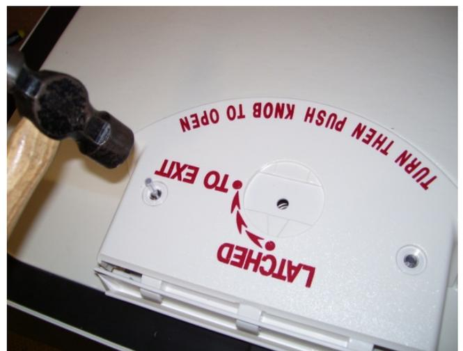
**STEP 12.** Hold the handle shield down against the lid. Insert the rivets into the holes in the shield and the holes in the lid. Lightly tap on the head of the rivets to set the rivets.
