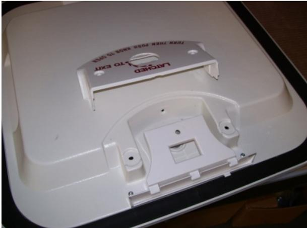
**STEP 5.** Remove the handle shield.
