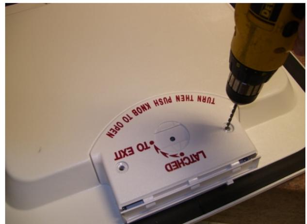
**STEP 4.** Using a 5/32" drill bit, carefully drill through the center of the plastic rivet. Remove both rivets.
