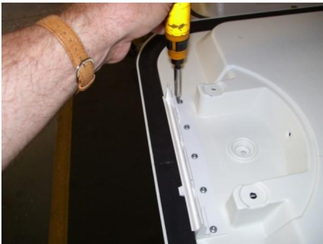
**STEP 7.** Using a T-20 Torx bit, remove the 5 screws that hold the handle base to the lid.
