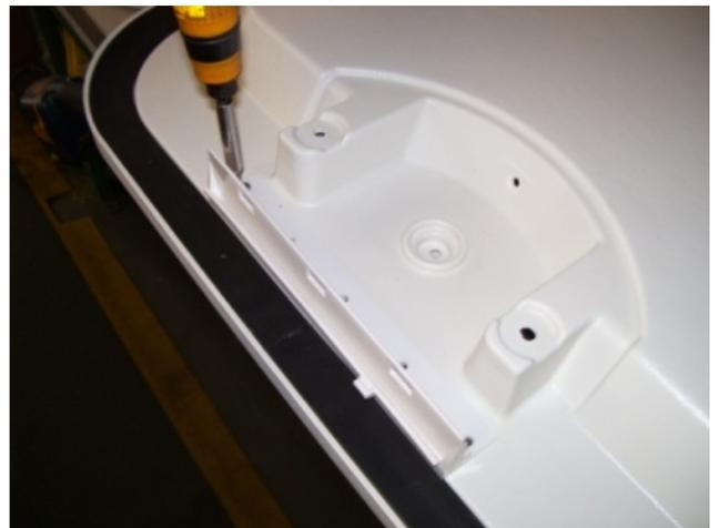
**STEP 8.** Using the same screws, attach the new handle base to the lid.
