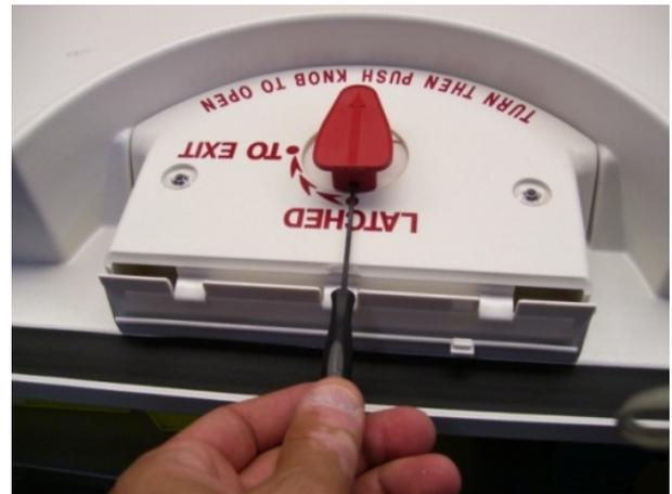
**STEP 2.** Orient the inner red knob as shown. Remove set screw in knob using 5/32" allen wrench.
