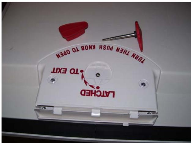
**STEP 3.** Unscrew the inner red knob from the outer red knob. Remove each from the lid.
