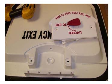
**STEP 5.** Remove the handle shield and inner knob components.
