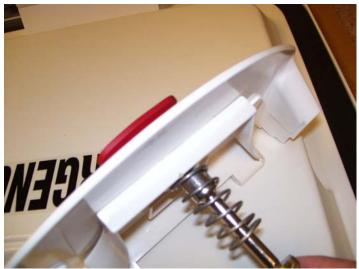
**STEP 8.** Replace the new handle into the subassembly. Rotate bolt 9.5 times for proper torque. The bolt should pass through each item in this order:
