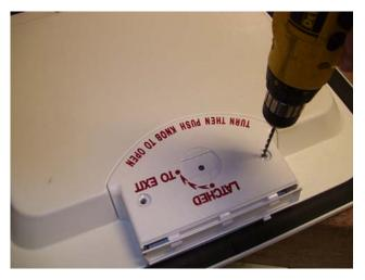
**STEP 2**. Using a 5/32" drill bit, carefully drill through the center of the plastic rivet. Remove both rivets.
