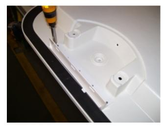
**STEP 10.** Using the same screws, attach the new handle base to the lid.
