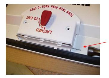
**STEP 12.** While pushing down on the handle shield, slide the hinge pin into the hole on the handle base. Pushing on the handle shield will help locate the pin during insertion. You will need to guide the pin into the second hole on the handle from underneath the handle. Lightly tap the pin with a hammer until the pin is fully inserted.
