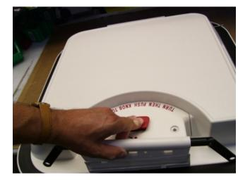
**STEP 1.** Remove the lid from the hatch frame (T-40 Torx drive). Place lid on a flat surface with the inside of the lid facing upward. Depress the inside red knob to remove release hinge.
