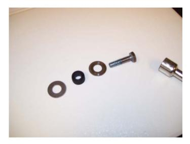
**STEP 7.** Remove the <sup>1</sup>/<sub>4</sub> Hex Bolt, (2) flat washers and rubber washer.
