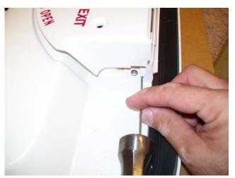
**STEP 3.** Lightly tap on the left hand end of the hinge pin (tapered end) until the opposite end is approximately 3/8" out of handle base.
