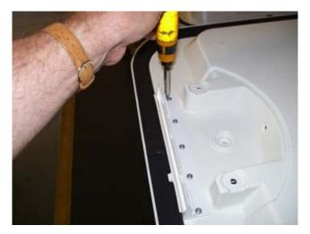
**STEP 9.** Using a T-20 Torx bit, remove the 5 screws that hold the handle base to the lid.
