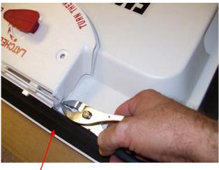
**STEP 4**. Remove the hinge pin from the side of the handle base. Pushing on the handle shield makes it easier to remove the pin. **Caution: gloves are recommended for this step as plastic edges can be sharp.** Rev1, 10-20-08
