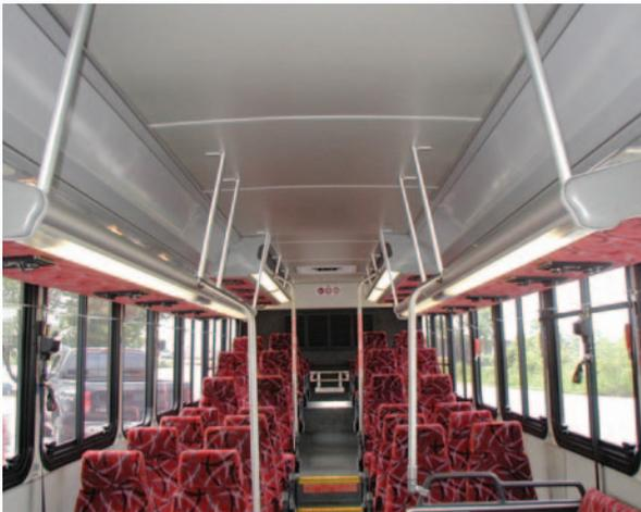
The SUBURBAN is a deluxe Overhead Parcel Rack (OPR) system with integrated HVAC duct as used in Suburban bus applications. The strong, yet lightweight, aluminum and steel construction of the SUBURBAN system provides spacious parcel storage as well as individual LED reading lights and A/C outlets in an attractive system specifically designed for every application.
