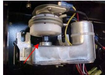
6. Position flats of motor shaft so that they are parallel to the base, for ease of assembly- then push into place as shown above. Reattach (2) each of washers, lock-washers and nuts to secure new motor in place.
