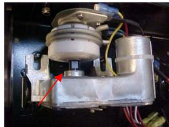
6. Position flats of motor shaft so that they are parallel to the base, for ease of assembly- then push into place as shown above. Reattach (2) each of washers, lock-washers and nuts to secure new motor in place.
