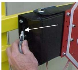
1. Using a utility knife, cut the silicone seal on both ends of the stop arm cover.
