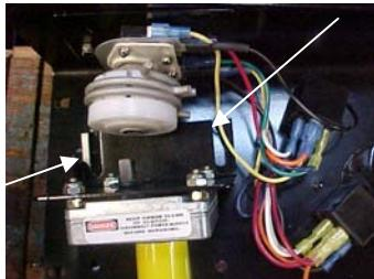
5. Remove (2) each of washers, lock-washers and nuts on the motor bracket and remove both the motor and bracket from the assembly, using a 7/16" socket
