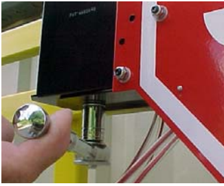
1. Remove 1/2-20 nut at the bottom of control box w/ 3/4" wrench.
