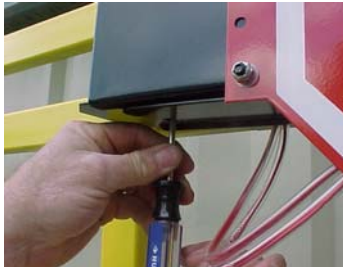
2. Use a screwdriver (or similar tool) to tap the cam shaft up inside the unit.
