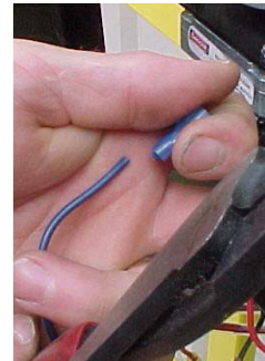
14. Cut Fast-On end off of BLUE wire, strip end approximately 1/4" & crimp new 1/4" fast-on blade, 004024, included with kit.
