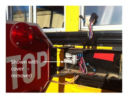
• Disconnect wiring (at weather pack or if wired directly) at old module. (picture above shows wired directly)
